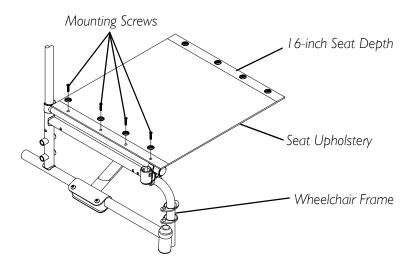
FIGURE 8.1 Replacing the Seat Upholstery
